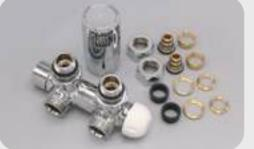
Angled valve block **TWIN VALVE** in chromed version with 50mm connection size, inlet is on the left side, including thermostatic head and compression fittings for 15mm copper and 16x2mm multilayer. **WITHOUT BYPASS**.
