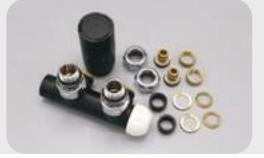
Angled valve block TWIN VALVE in color Soft Black with 50mm connection size, inlet is on the right side, including thermostatic head and compression fittings for 15mm copper and 16x2mm multilayer. WITHOUT BYPASS.
