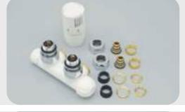
Angled valve block TWIN VALVE in color Soft White with 50mm connection size, inlet is on the right side, including thermostatic head and compression fittings for 15mm copper and 16x2mm multilayer. WITHOUT BYPASS.
