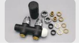
Straight valve block TWIN VALVE in color Soft Black with 50mm connection size, inlet is on the right side, including thermostatic head and compression fittings for 15mm copper and 16x2mm multilayer. WITHOUT BYPASS.
