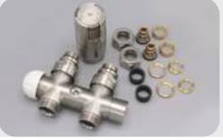
Straight valve block TWIN VALVE with brushed stainless steel look with 50mm connection size, inlet is on the right side, including thermostatic head and compression fittings for 15mm copper and 16x2mm multilayer. WITH BYPASS.
