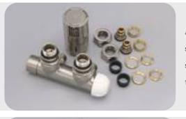
Angled valve block TWIN VALVE with brushed stainless steel look with 50mm connection size, inlet is on the right side, including thermostatic head and compression fittings for 15mm copper and 16x2mm multilayer. WITH BYPASS.
