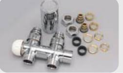
Straight valve block **TWIN VALVE** in chromed version with 50mm connection size, inlet is on the right side, including thermostatic head and compression fittings for 15mm copper and 16x2mm multilayer. **WITHOUT BYPASS**.
