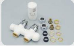
Straight valve block TWIN VALVE in color Soft White with 50mm connection size, inlet is on the right side, including thermostatic head and compression fittings for 15mm copper and 16x2mm multilayer. WITHOUT BYPASS.
