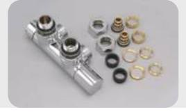
Angled valve block **TWIN VALVE LIGHT** in chrome finish with a 50mm connection size. The inlet is located on the right side, without a bypass, and equipped with compression fittings for 15mm copper and 16x2 multilayer pipes.
