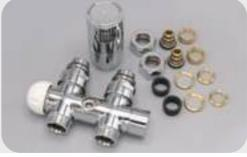
Straight valve block **TWIN VALVE** in chromed version with 50mm connection size, inlet is on the right side, including thermostatic head and compression fittings for 15mm copper and 16x2mm multilayer. **WITH BYPASS**.
