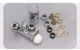
Terminal block **SWITCH**, by adjustable connections both can be used at right angles as straight, in chromed version, with 50mm connection size, including thermostatic head and compression fittings for 15mm copper and 16x2mm multilayer. WITHOUT BYPASS.
