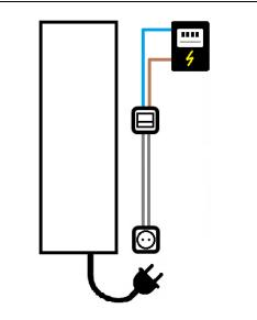
Create a situation where the contact point for the electric radiator (e.g. socket) has a direct connection to the mounting box where the thermostat will be installed. From this mounting box follows the connection to the power.
